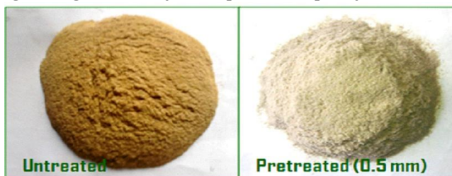
Fig. 2: Physical appearance of paddy straw before and after alkali treatment
