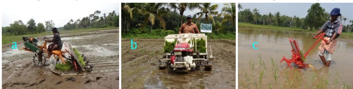
Fig. 1: Different types of planters used in present study: a) Redlands 8 - row riding type, b) Mahindra 4 row walking type, and c) Manual 2 row transplanter
