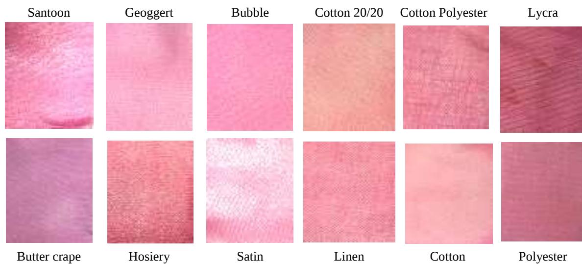
Fig. 3: Dyed fabrics samples after washing (acidic pH)
