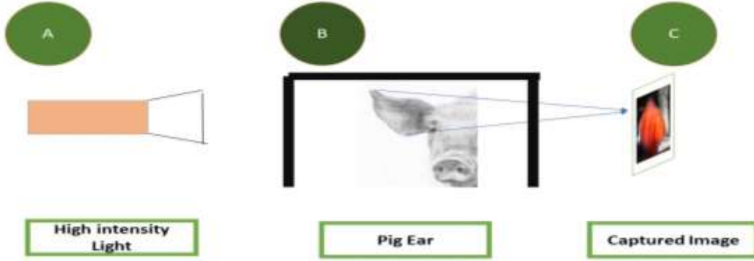
Fig. 1: Image acquisition; A) High intensity light has projected on the ear leaf of pig, B) Pig ear placed in box, and C) Captured image of ear leaf with proper vein web on the other side of ear using mobile phone
